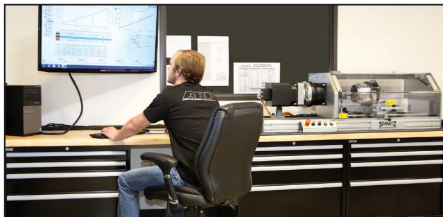
ARP's computer-controlled torque-tension machine can apply a given "torque" or "angle" to a fastener and measure the actual preload. Through test cycles, it is possible to chart the "preload scatter" with various fasteners and lubricants.
